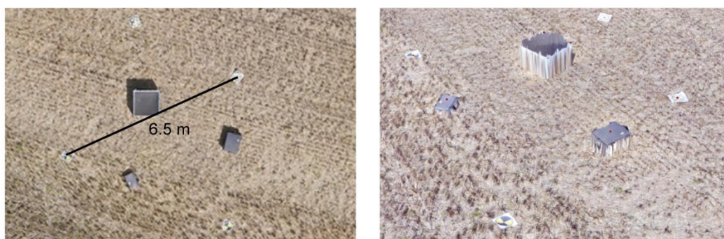
Figure 4-8: Experimental design of accuracy assessment (left: photo, right: DEM): Reference points are four GCPs, two different sized Peli Cases and 4 corners of the UAV transport box.
