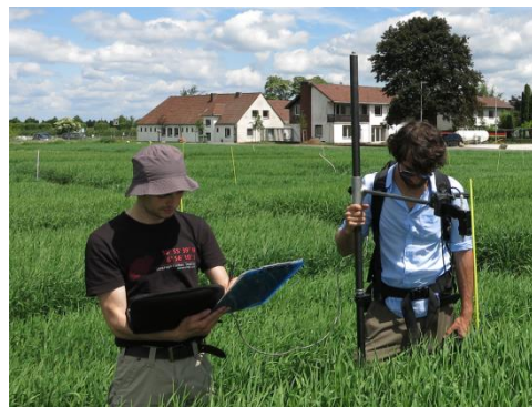
Figure 7-2: Sampling hyperspectral ground truth with an ASD FieldSpec3.
