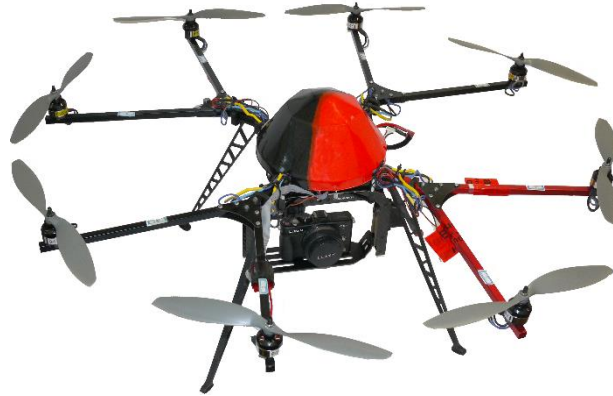
Figure 3-3: MK-Okto by Hisystems GmbH mounted with Lumix DMC GF3 optical camera (BENDIG ET AL., 2013).
