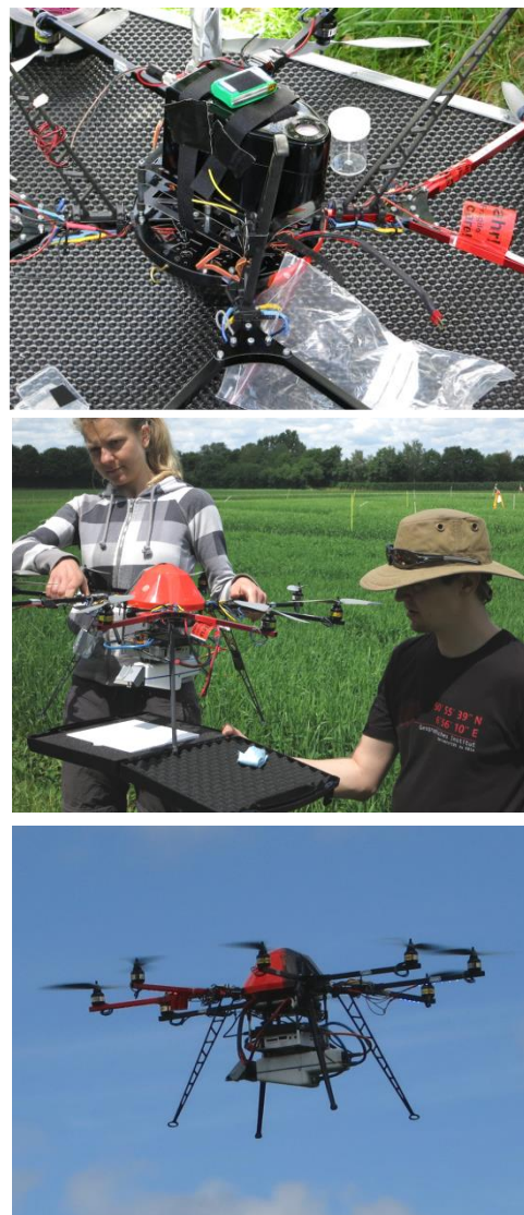
Figure 7-1: top: MK Oktokopter is prepared for a flight campaign with the Rikola Hyperspectral Camera, middle: Cubert UHD185 Firefly is calibrated against a white panel before take-off, bottom: UHD185 in the air mounted on a MK Oktokopter.
