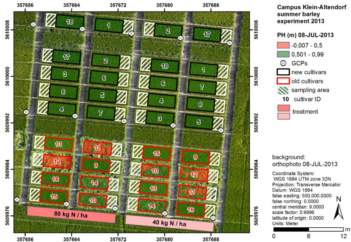
Figure 8-6: Lodging detection based on PH at the summer barley study site Campus Klein-Altendorf, Rheinbach, 08 July 2013, GCPs = ground control points used for CSM generation.
