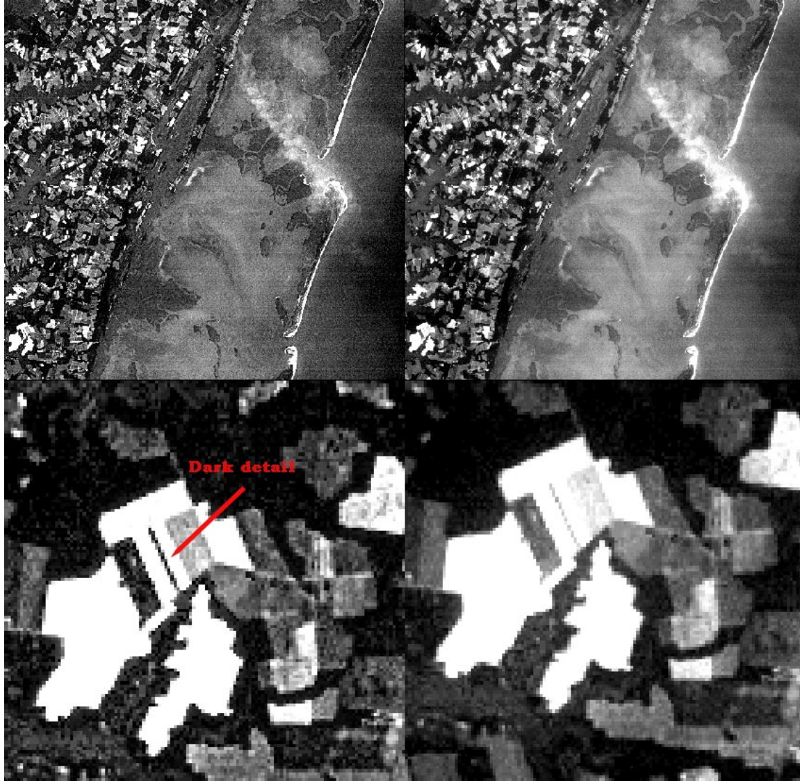
Figure 10: Comparison of TM band 1 data corrected for atmosphere (left side) to uncorrected counts (right side). The correction includes adjacency effect correction.
