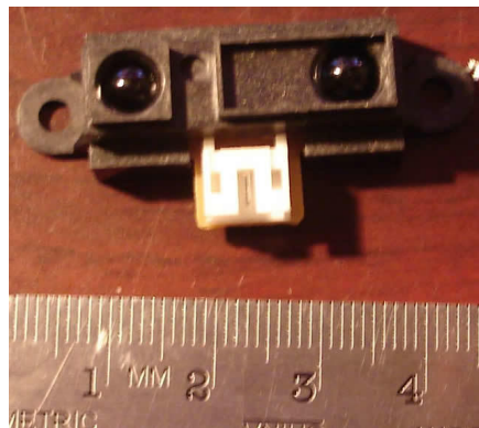
Figure 31 A Sharp GP2D120 infrared range sensor
