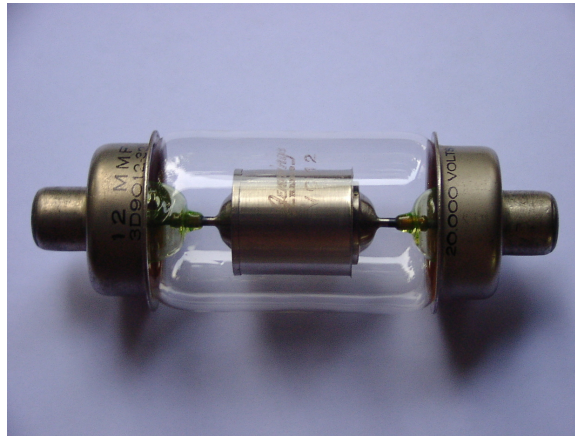
Figure 72 Vacuum capacitor with uranium glass encapsulation
