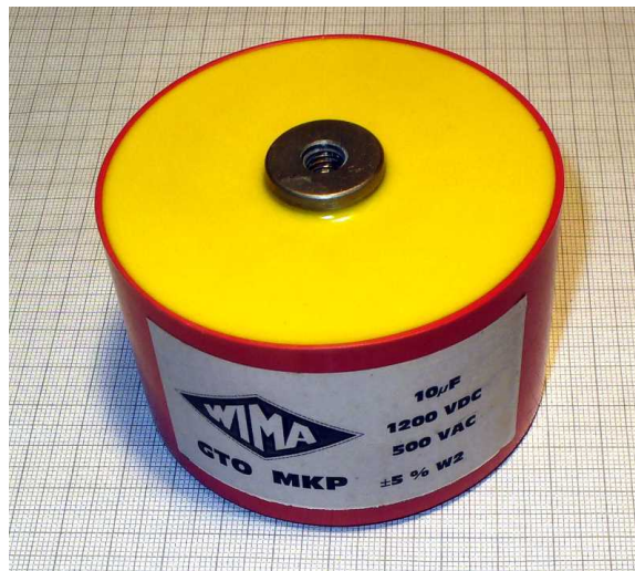
Figure 53 Heavy-duty snubber capacitor with screw terminals
