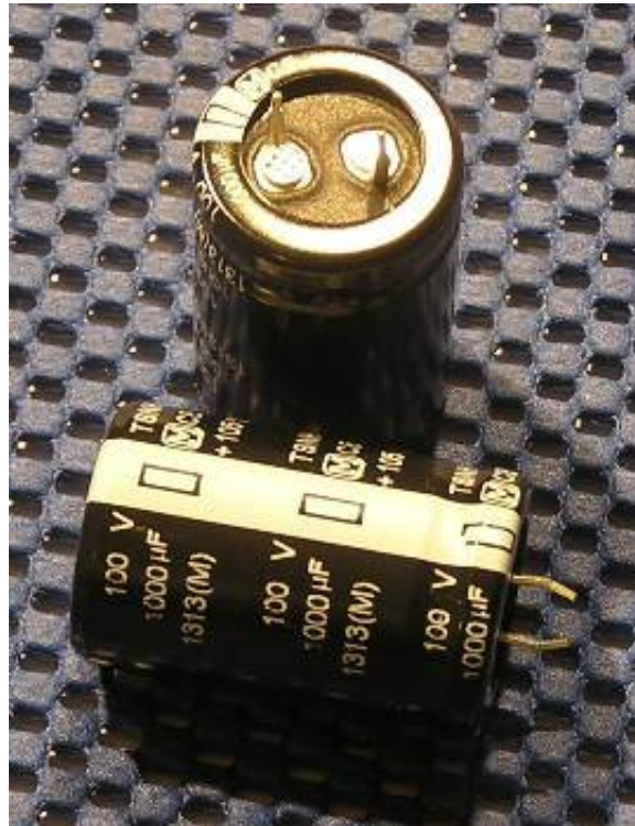
Figure 62 Snap-in style of aluminum electrolytic capacitors for power applications
