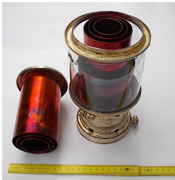
Figure 74 Vacuum tuning capacitor
