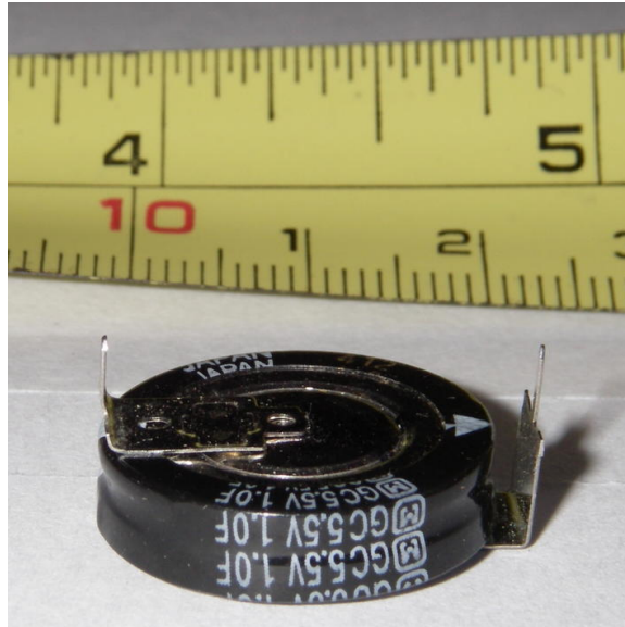
Figure 68 Double-layer capacitor with 1 F at 5.5 V for data buffering
