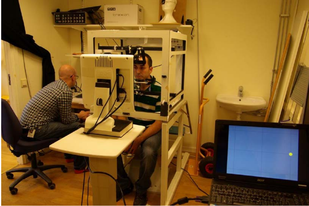
Figure 3.1: The scleral search coil setting. Picture taken at Bernadottelaboratoriet at S:t Eriks Ögonsjukhus during the Tobii Alignment validation against SSC technique.
