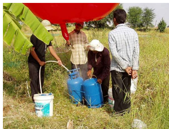
Fig 2: Balloon filling with Hydrogen Gas
