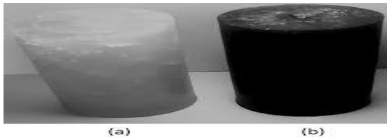
Figure4: Photograph of (a) pure paraffin as PCM and (b) Paraffin/graphite composite
