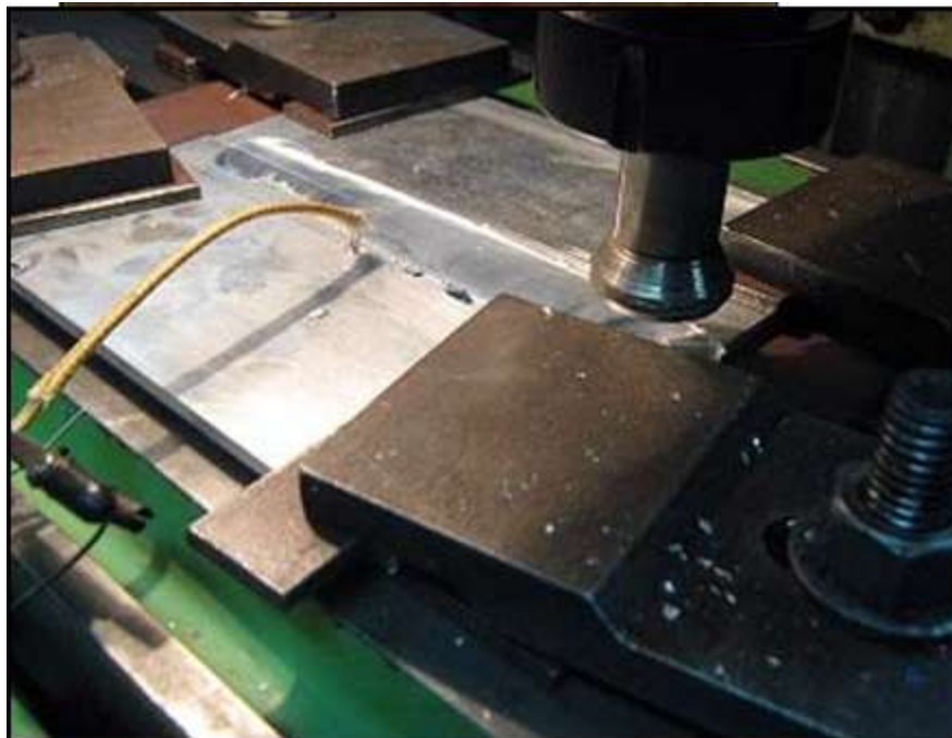
Figure 3.14: FSW of aluminum plate in progress.
