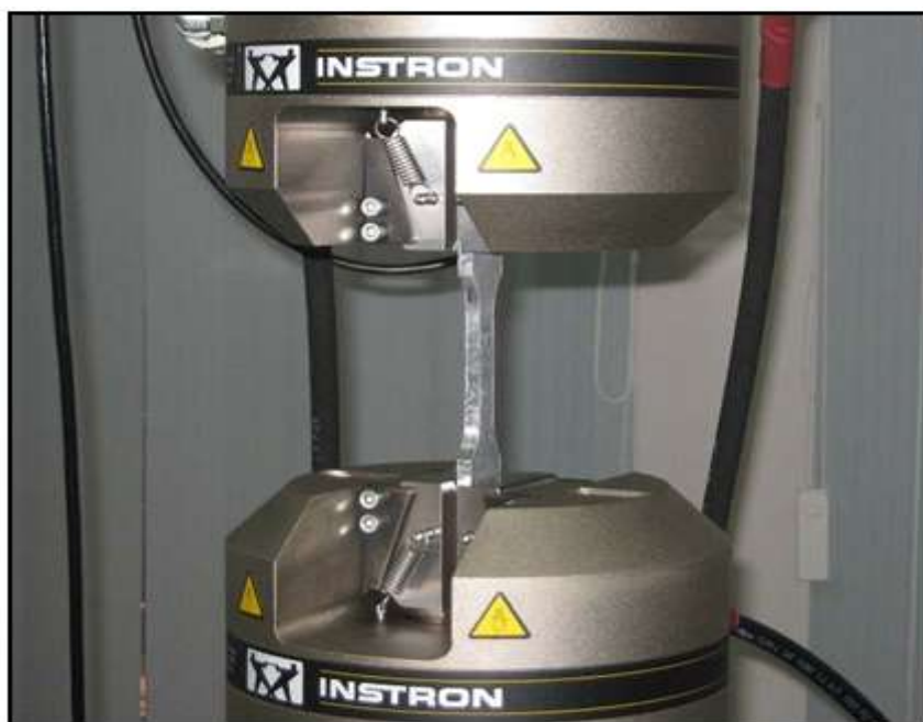
Figure 3.9: Close-up view of tensile testing of FSW Joints.
