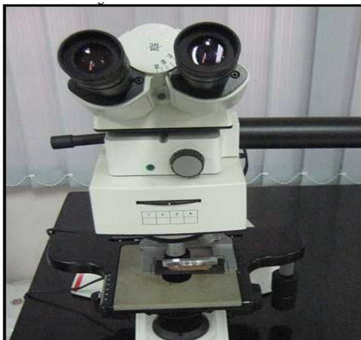
Figure 3.11: Metallographic testing of FSW joints.
