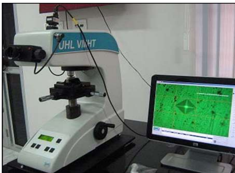
Figure 3.12: Metallographic (hardness) testing of FSW joints.
