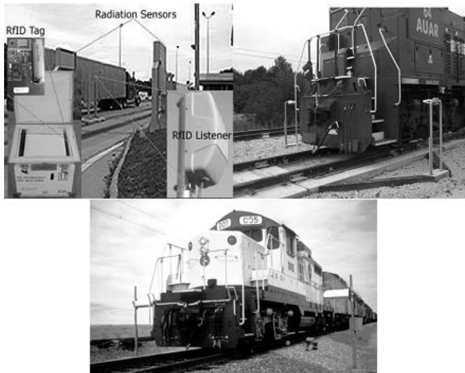
Figure 8 - Examples of automatic readers that can be installed for rail and road transport
