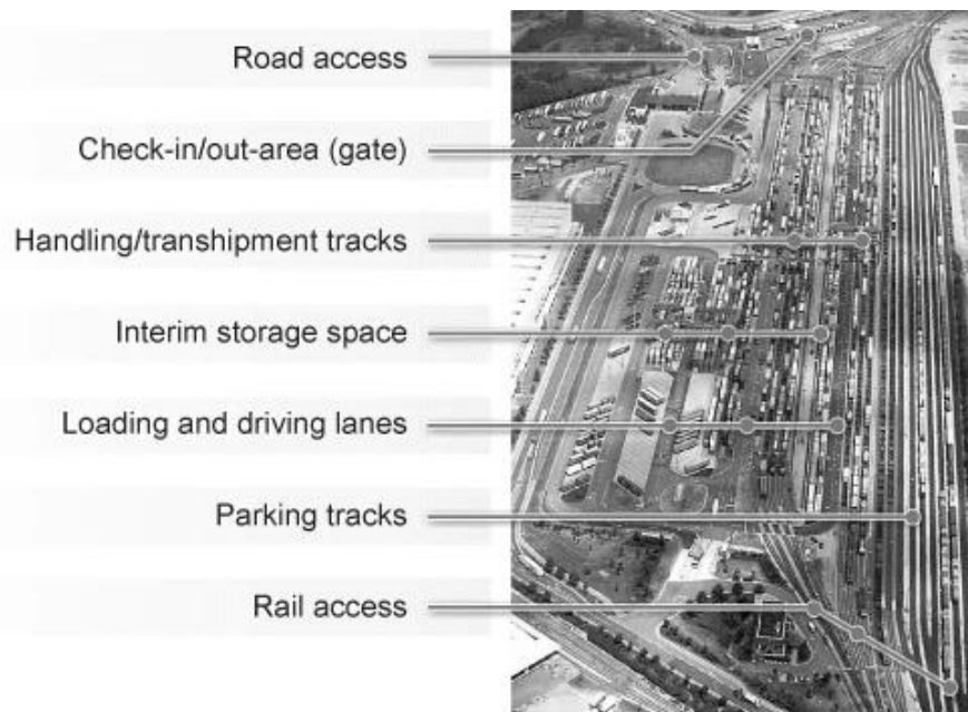
Figure 3 - Road-rail terminal module (Intermodal Terminals, 2012)
