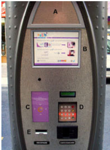
Figure 7 A Vélib' station kiosk
