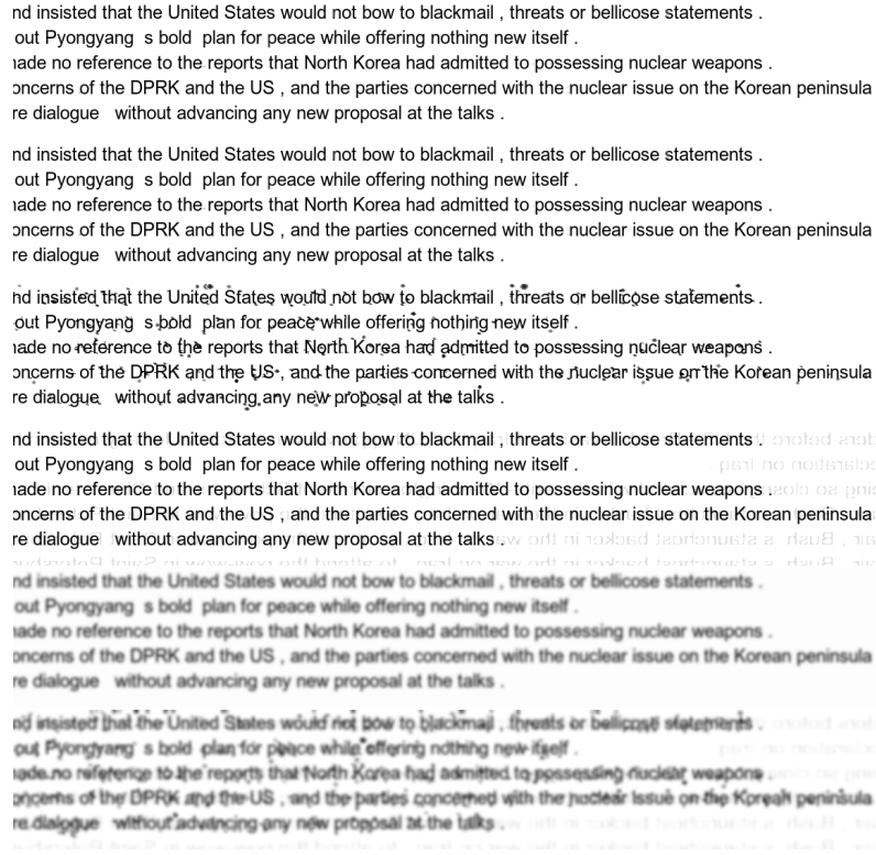
Fig. 2. Example of types of noise applied on a dataset: (i) clean image, (ii) Phantom Character , (iii) Character Degradation , (iv) Bleed Through , (v) Blur , and (vi) all mixed together.
