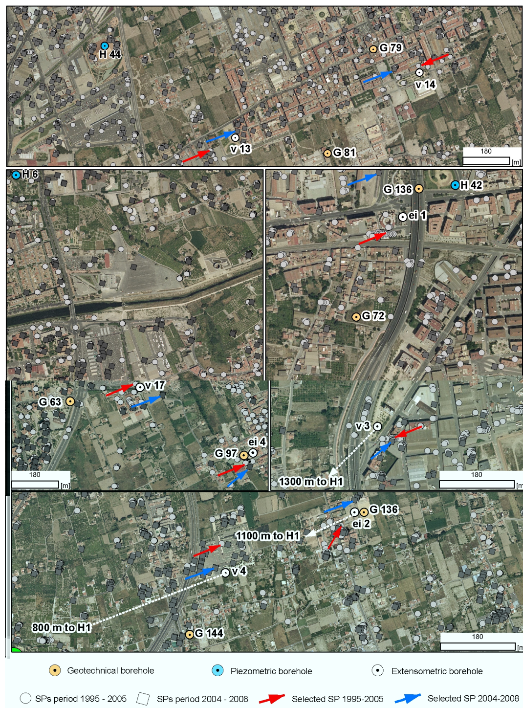
Fig. 6. Location of the selected SPs around each extensometer. The white arrow indicates the distance to the closest piezometer.
