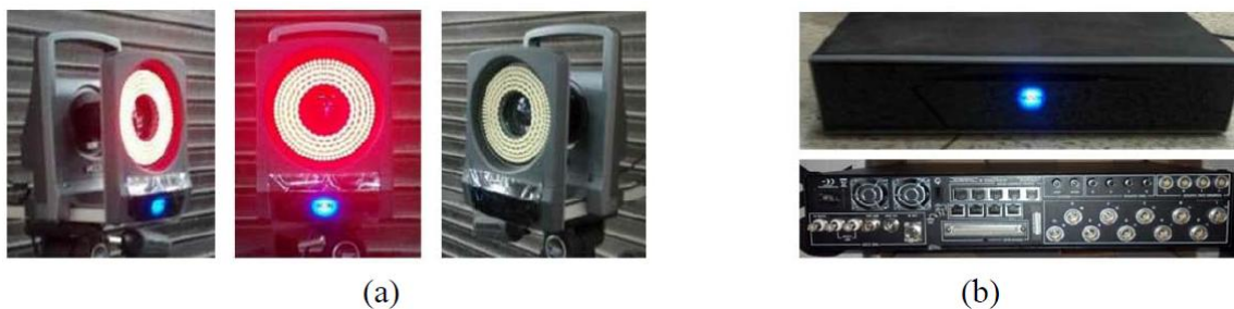
Figure 1. Motion-capture system. (a) Camera; (b) Vicon giganet.
