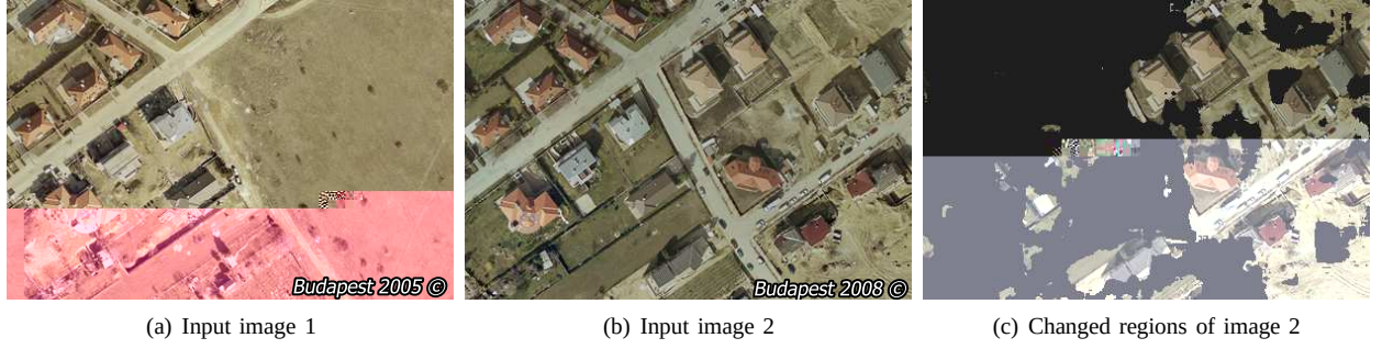
Fig. 6. Low level change detection: (a) and (b) input images, (c) Bhattacharyya change mask P_{ch}
