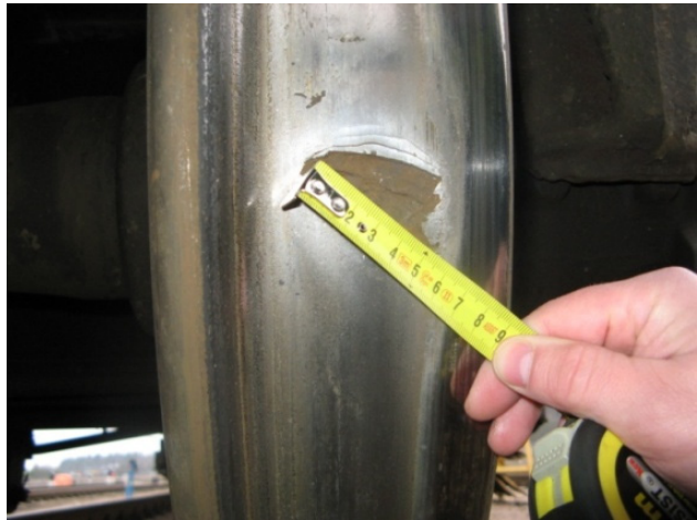
Fig. 7. Crack length measuring with a ruler.
