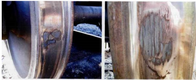
Fig. 2. Inadmissible wheel flat on the wheel rolling surface.
