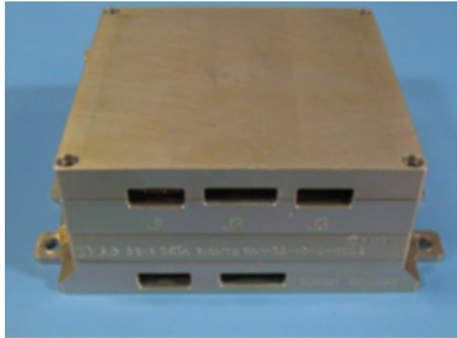
Figure 11: CSR-SDR-S/S radio. (Courtesy of Vulcan Wireless Inc.)
