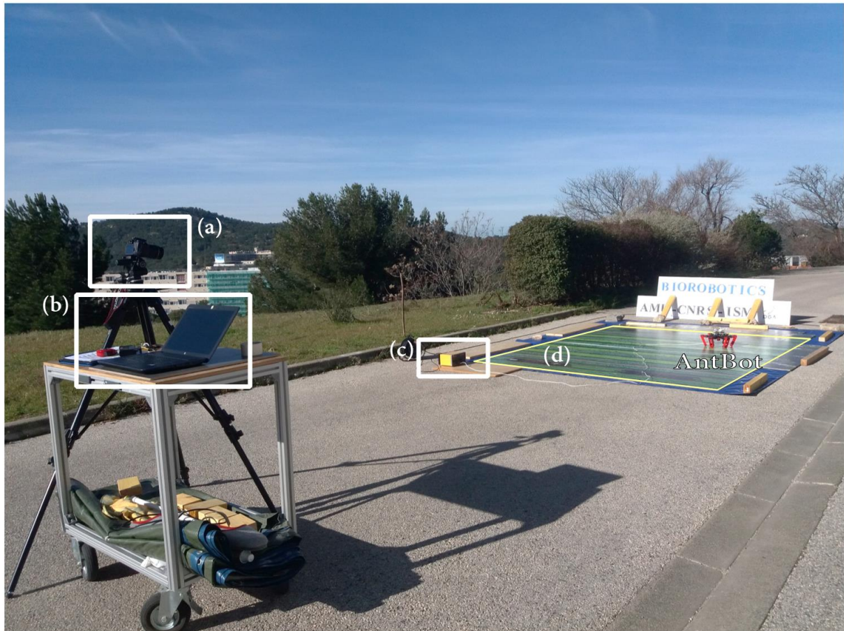
Fig. S9. Photograph of the experimental setup. AntBot navigates on a textured panel measuring 3m x 4m (d), powered by the DC generator (14V, 10A) shown in (c). The ground-truth was acquired using the high-resolution reflex camera (Canon EOS 650D) presented in (a). The experiments were managed with the host computer (b).
