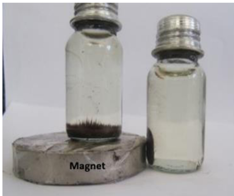
Fig. 3 Demonstration of magnetic separation at 30 s
