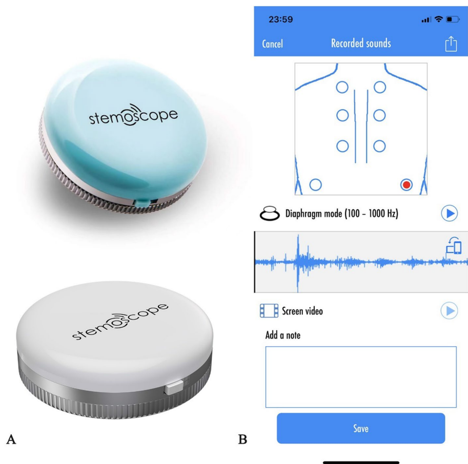
Fig. 4 A Stemoscope. B Stemoscope App to record the respiratory sounds. Tap the red dot on the screen to start recording the sounds. Then the investigators can play the recorded sounds. The App provides powerful options to share recorded sounds, such as Twitter, Facebook, and WeChat
