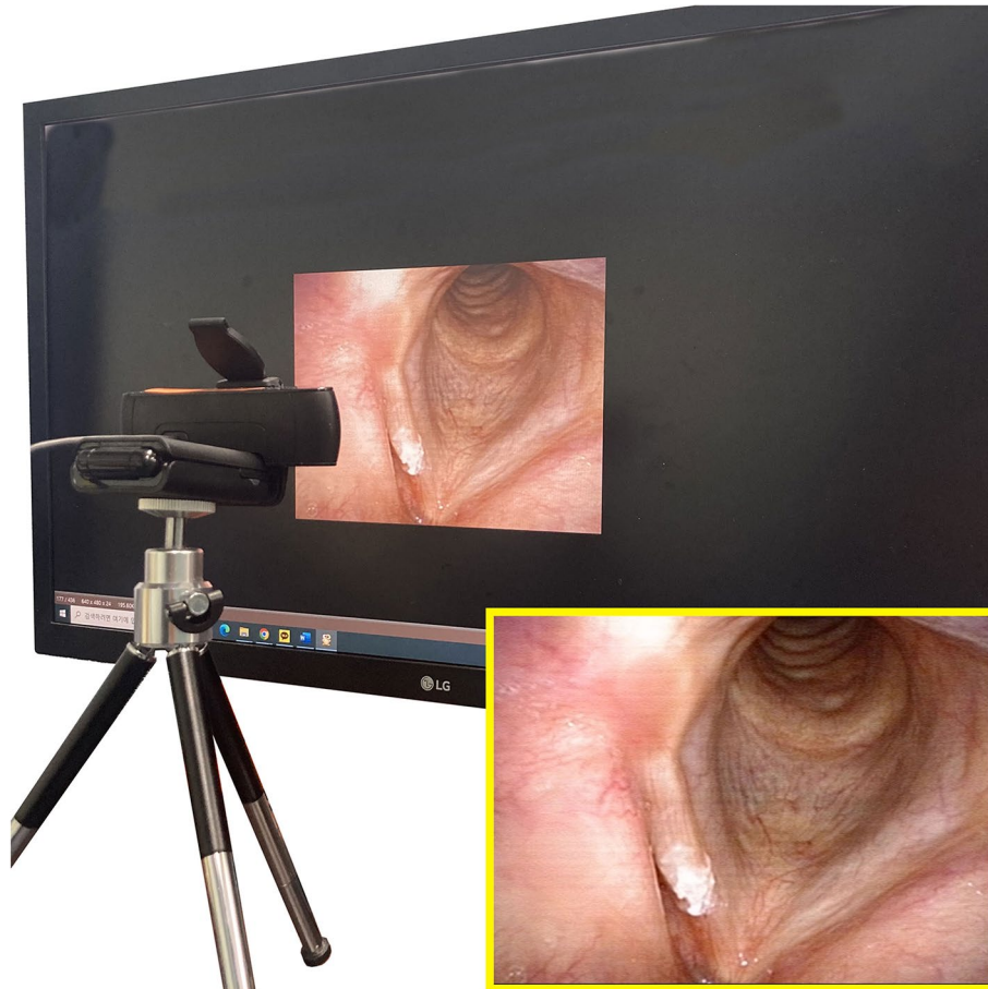
Fig. 7 Evaluation of the embedded-ported convolutional neural network model using a web camera. The image in the yellow rectangular contour represents the web camera-photographed image
