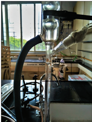
Figure 1: Collection of essential oils by Clevenger Apparatus
