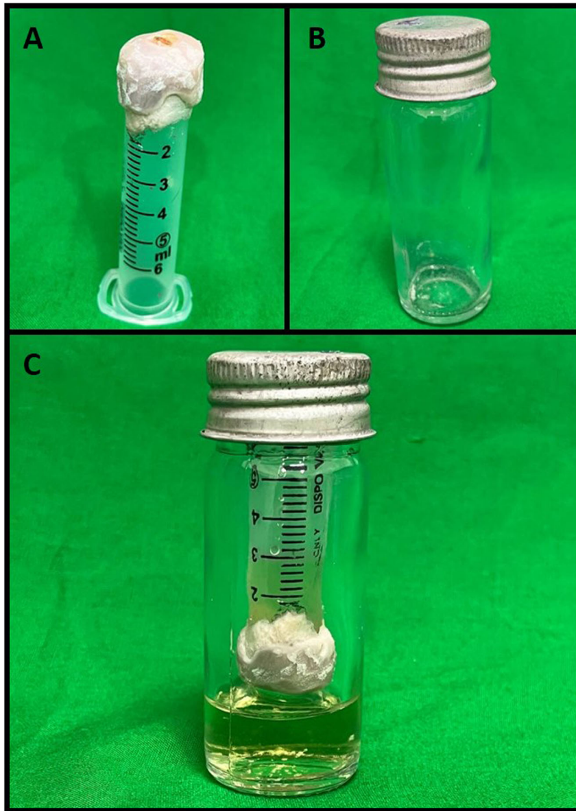
Fig. 3 The bacterial microleakage apparatus. A The upper chamber of the apparatus was prepared using a plastic syringe and acrylic. The tooth is inserted such that the apical end is exposed. B The lower chamber of the apparatus- McCartney bottle. C The apparatus assembled together with sterile Muller Hinton broth in the lower chamber and upper chamber inoculated with E. faecalis .
