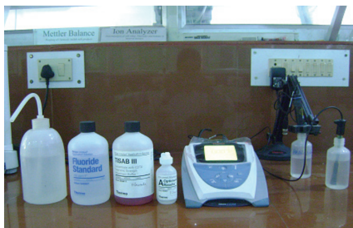
[Table/Fig-1]: Fluoride ion selective electrode (Orion-9609BNWP) coupled to an ion analyzer used for measurement of Fluoride ion concentration
