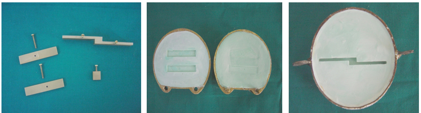
[Table/Fig-2]: Brass dies used in the study [Table/Fig-3]: Moulds prepared for acrylic resin strips [Table/Fig-4]: Mould prepared for making shear bond strength samples
