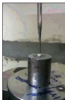
[Table/Fig-1]: Specimen mounted on universal testing machine [Table/Fig-2]: Extrusion of filling material
