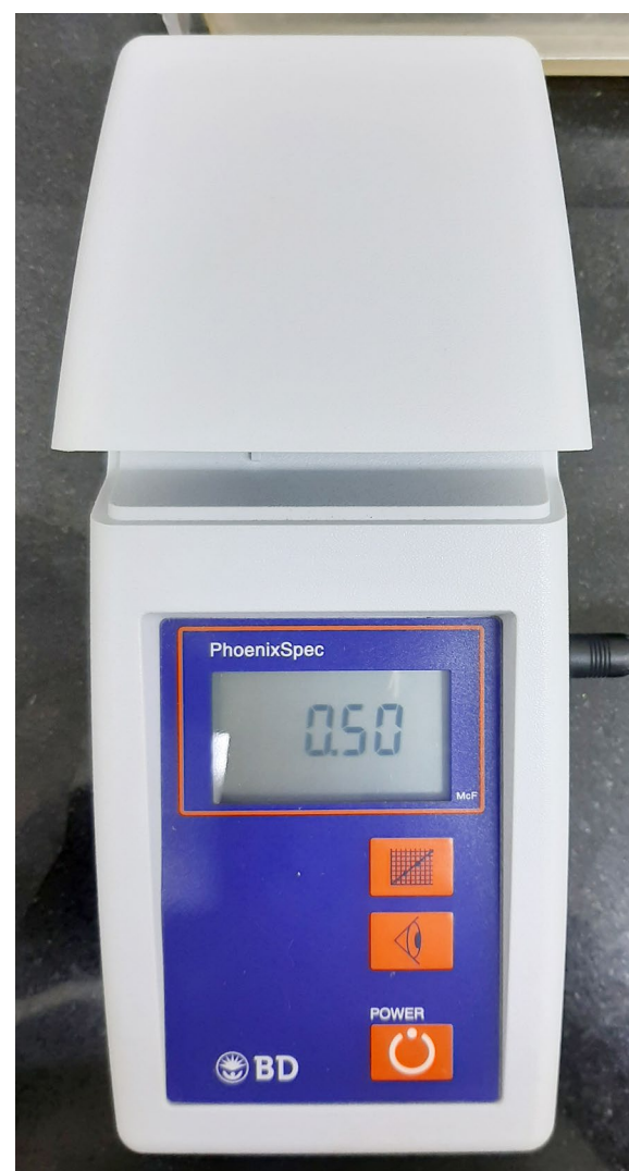
Fig. 5 The BD PhoenixSpec™ nephelometer for reading the mcfarland standard
