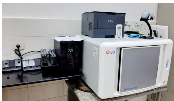
Fig. 4 BD Phoenix™ automated identification and susceptibility testing system
