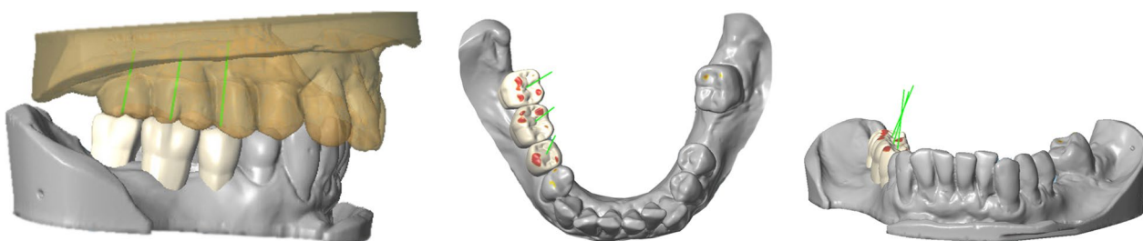
Fig. 5 Prosthetic set-up in a full CAD-software (Cares, Dentalwings) using individual tools to create restorations and adapt the occluding surfaces
