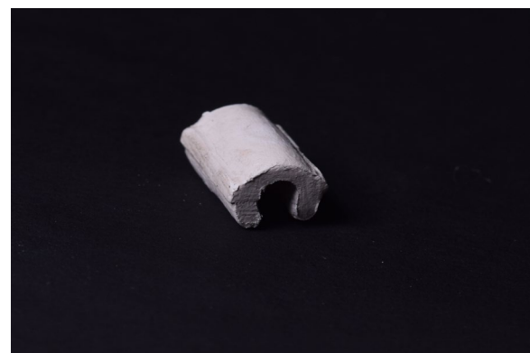
Fig. 4 Pressed PEEK clip
