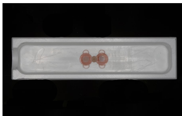
Fig. 2 The brushing container, in which the samples were covered with the respective toothpaste slurry and subjected to the brushing sequence
