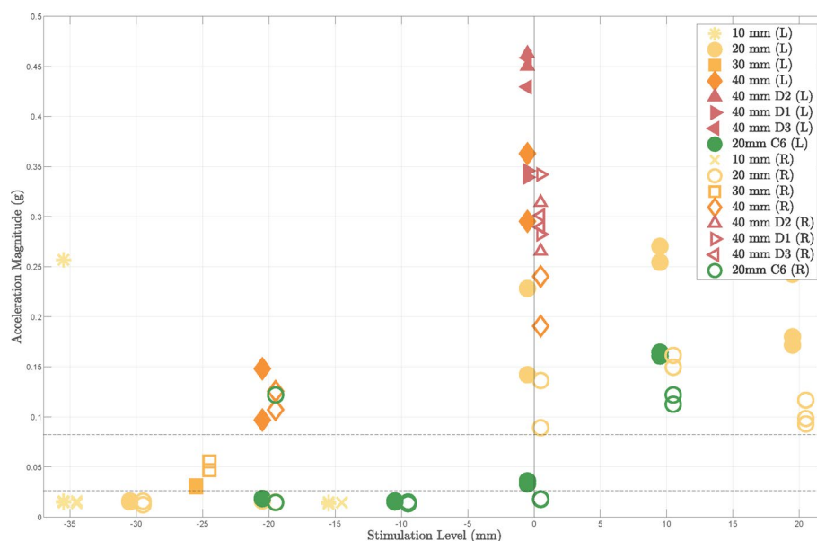
Fig. 7 Left (L, filled markers) and right (R, empty markers) acceleration amplitude as a function of the esophageal stimulation level around rib 1 (orange-shades) and C6 (green) as well as the electrode spacing (10–40 mm) with a stimulation intensity of 40 mA. The average left and right acceleration amplitude achieved during stimulation with the needle electrode is indicated as an upper and lower dashed line, respectively. Compared to impulses from the needle electrode, significantly higher acceleration values are measured through stimulation with esophageal electrodes at the level of rib 1, which are as attributed to a higher amount of co-stimulation
