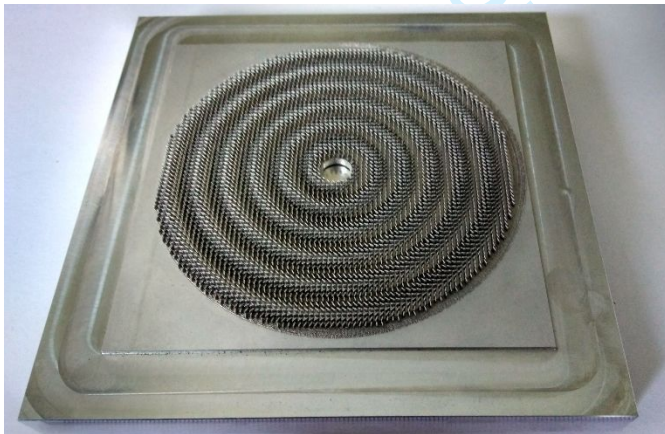
Fig. 7. Metal-only RHCP Ka-band metasurface antenna [15].
