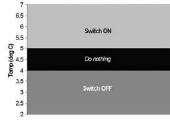
Fig. 5. Normal operating strategy of a refrigerator
