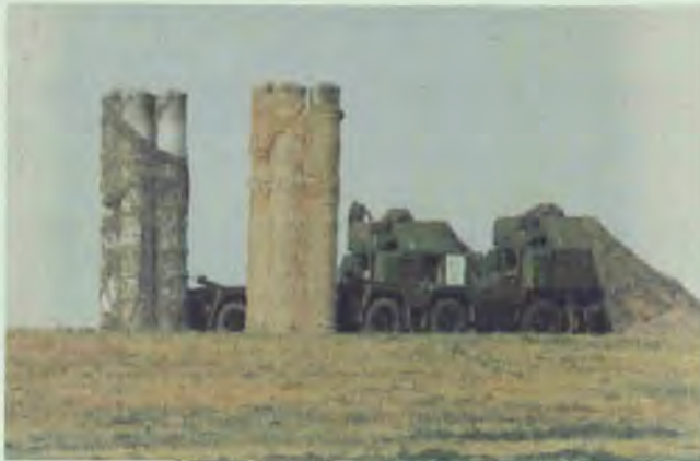
The Soviet Union has begun deployment of newly modernized surface-to-air missiles — SA-10s — which have the ability to engage several targets simultaneously, with increased firepower. Soviet SAMs provide barrier, area, and point air defense.
