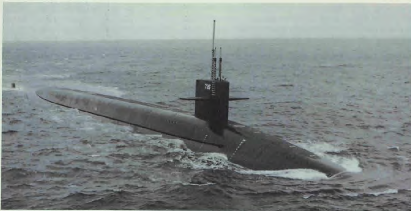
The Ohio-class ballistic missile submarine is now armed with the new Trident II (D-5) missile. The Trident II delivers a larger payload than current SLBMs, with significantly improved accuracy, at a nominal range of 7,400 km. Nine of these boats are operational, and eight others are in various stages of construction.
