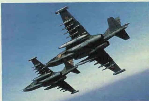
A pair of Su-25 Frogfoots, the Soviet Air Force's twin-engine, subsonic, close air support fighter, banks across the horizon. The aircraft, used also in short-range interdiction missions, is armed with air-to-ground ordnance, including antitank rockets and missiles, and an internal twin-barrel 30-mm gun.
