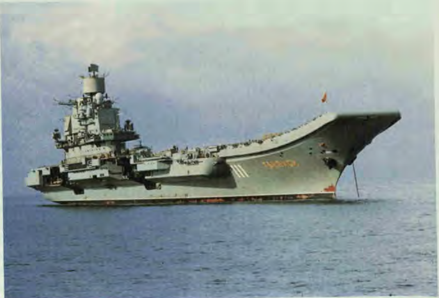
The sweeping, ski-jump bow of the new Tbilisi-class aircraft carrier makes it the first class of Soviet carriers capable of over-the-bow launches of conventional, fixed-wing aircraft. The Tbilisi carries 12 SS-N-19 long-range, vertically launched antiship missiles forward with flush-deck missile hatches on the bow deck.
