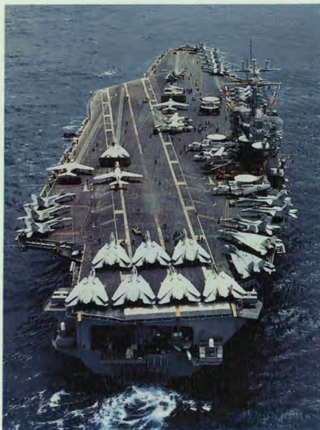
The nuclear-powered aircraft carrier USS Theodore Roosevelt (CVN-71) carries an air wing of 89-90 aircraft including fighter squadrons, light attack squadrons, medium attack squadrons, antisubmarine-warfare and electronic-warfare aircraft, early-warning aircraft, and ASW helicopters.
