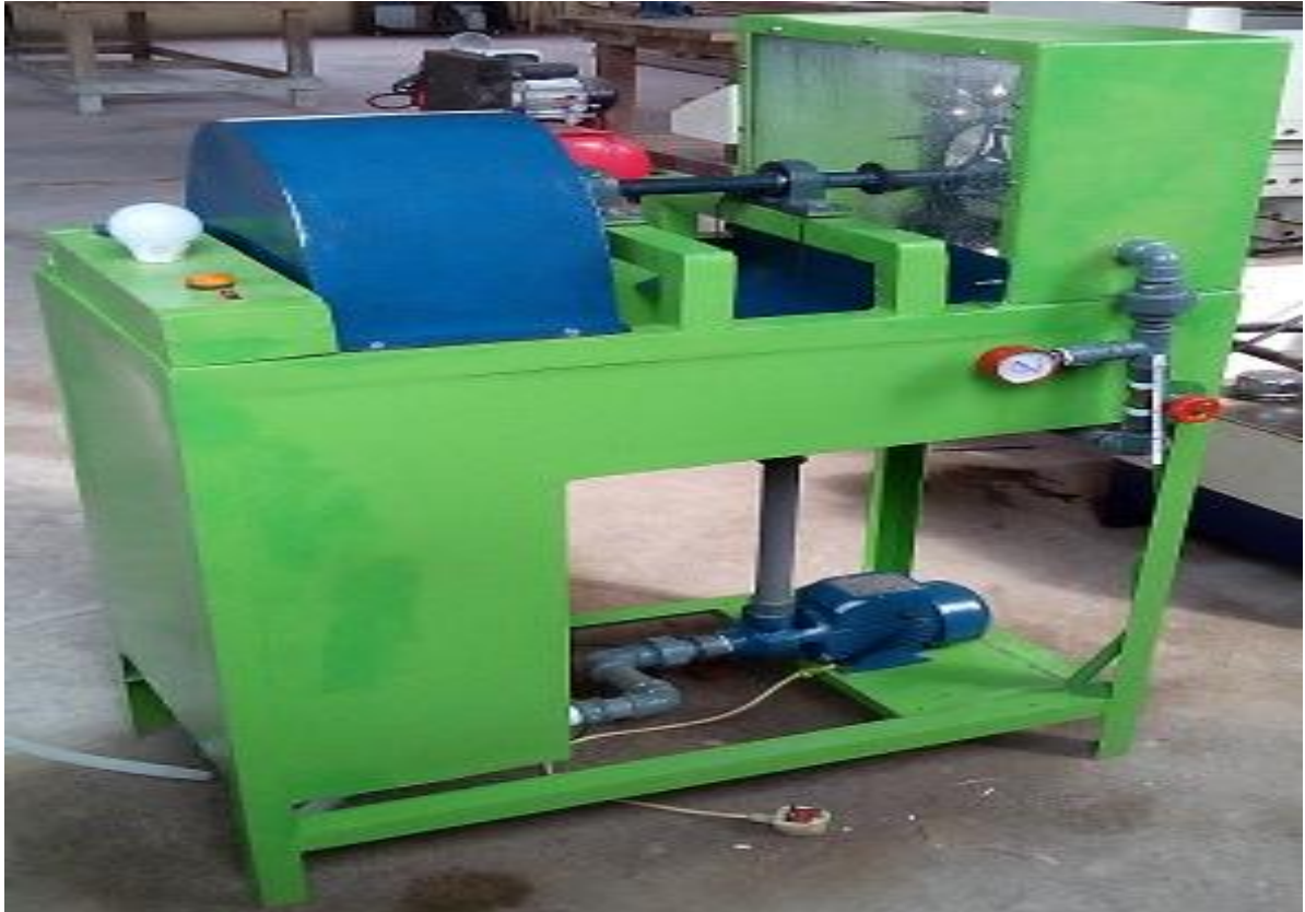
Figure 3.4: The Manufactured Pelton wheel (Impulse Turbine) in Akwalbom State University's Workshop
