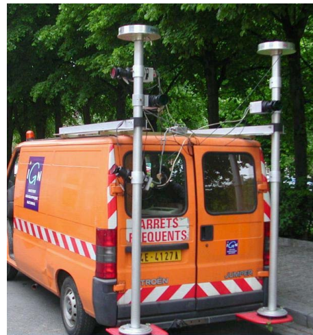
Figure 1: One vertical baselines of the Stereopolis system.
