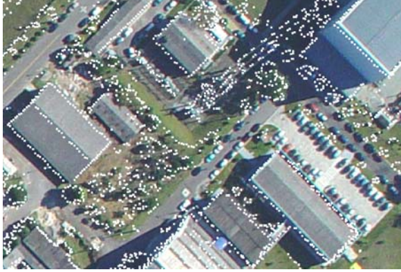
Picture 02 – Shows the laser scanner points selected in the region with big buildings
