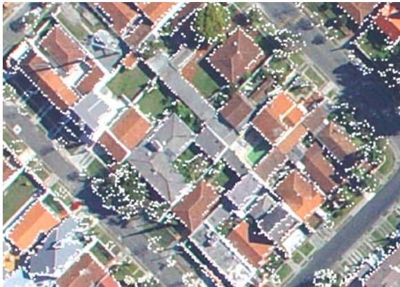
Figure 3: Shows the laser scanner points selected in the region of small buildings.
