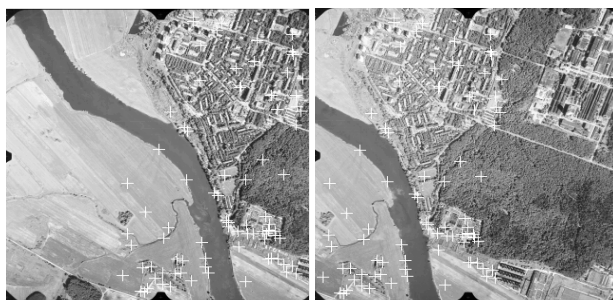
Figure 11. Accepted conjugate points, automatic relative orientation of aeroborn images
