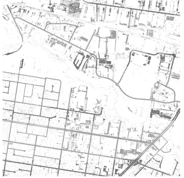
Figure 5: The road candidate points after intensity filtering.
