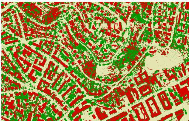
Figure 4.5- Results of the final classification of combining the road method with the robust method - site No. 2.
