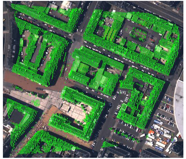
Figure 4: Laser points (in green) classified as non-ground points projected onto an aerial image (20 cm resolution) over the city of Amiens, France.
