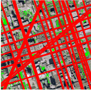
Figure 4. Road stripe detection by Hough transform from segmented lidar data
