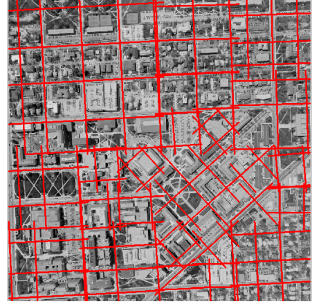
Figure 8. Detected lines on the road by acupuncture method
