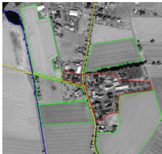
Figure 7. Extracted line and area features from an orthophoto
