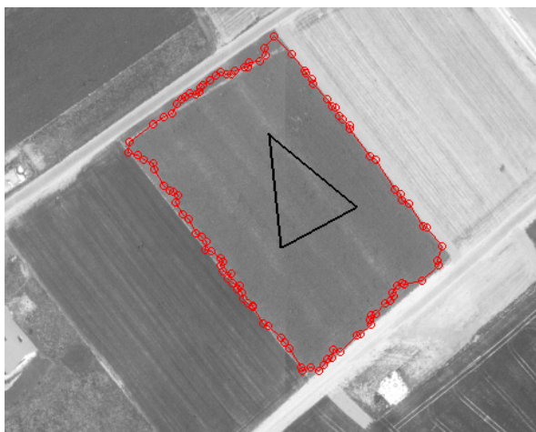
Figure 3. Parcel extraction example with starting polygon (black) and extraction result without smoothing (red)
