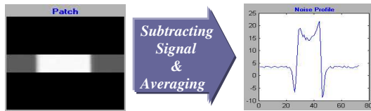
Figure 7. Left: Signal profile (result of lowpass filter), Right: Noise profile.
