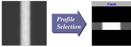
Figure 5. One of the edge targets (left) and corresponding picked up patch
