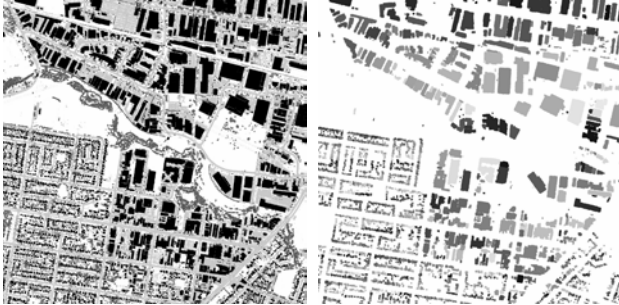
Figure 1. Left: results of the initial classification. White: grass land. Light grey: bare soil. Dark grey: trees. Black: buildings. Right: the final building label image.
