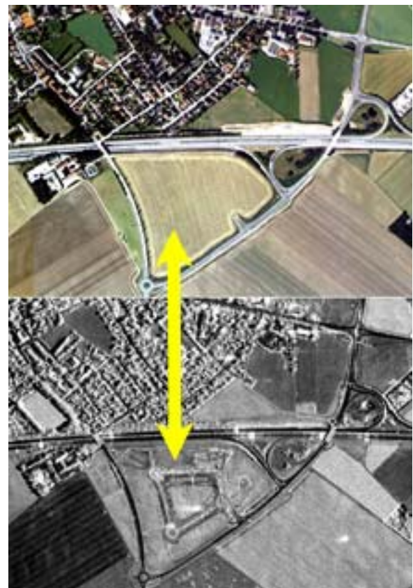
Figure 2: Comparison of optical and SAR images
