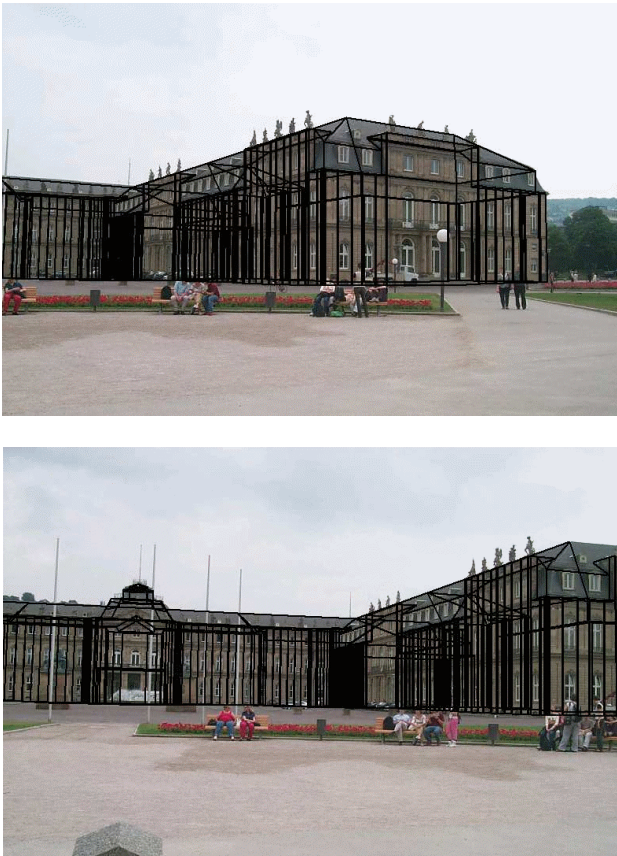
Figure 8: Wire-frame model mapped to different images
