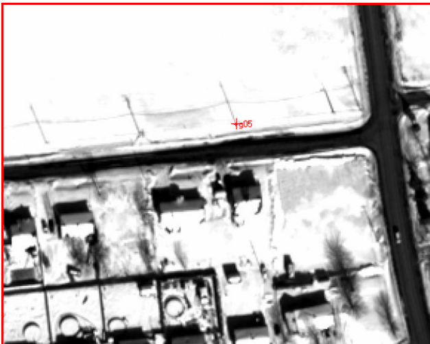
Figure 3. Example of GCP collected with hand-held GPS: the pole defined with its shadow. Even the shadow of the power line is visible on the snow. QuickBird © 2002 and Courtesy DigitalGlobe.
