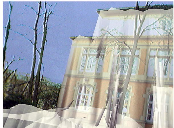
Figure 6. Superposition of video and laser-scanning model
