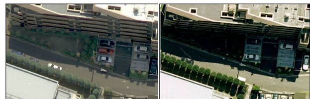
Figure 14. Example showing the difference in color depth of shaded area between DMC (left side) and filmed camera (right side)
